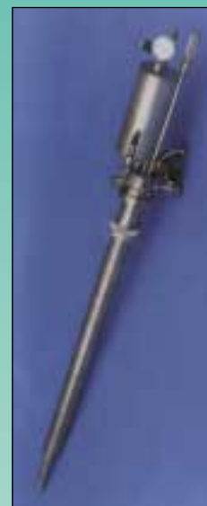
Bottom loading ^3\text{He} unit.
