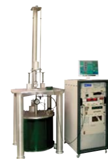
16 Tesla cryogen free measurement system
