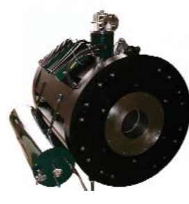
6.5 Tesla iron shielded magnet for Nuclear beam experiments
