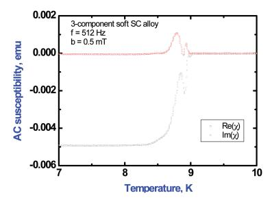
Temperature dependence of the AC susceptibility of a superconducting alloy
