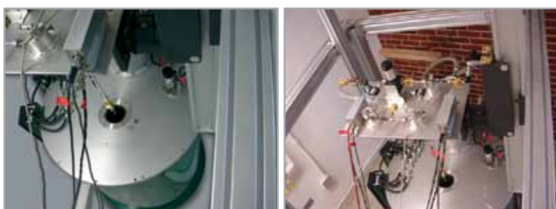
High performance W-band microwave bridge installed above 12 T cryogen-free magnet (courtesy Dr. A. Smirnov, North Carolina State University)
