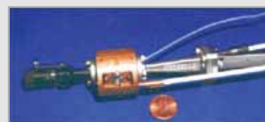
Probe head for W-band EPR (above) and associated resonator (below) with sample tube highlighted by arrow (courtesy Dr. A. Smirnov, North Carolina State University)
