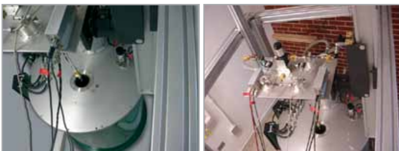
High performance W-band microwave bridge installed above 12 T cryogen-free magnet (courtesy Dr. A. Smirnov, North Carolina State University)
