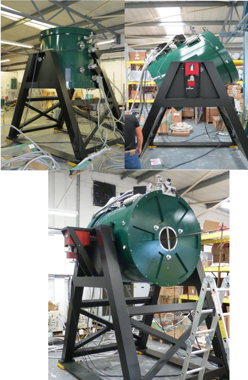
Figure 1: Photographs of 5 T magnet system with 300 mm bore. Rotation frame allows the field orientation to be controlled between horizontal and vertical with 1° accuracy.
