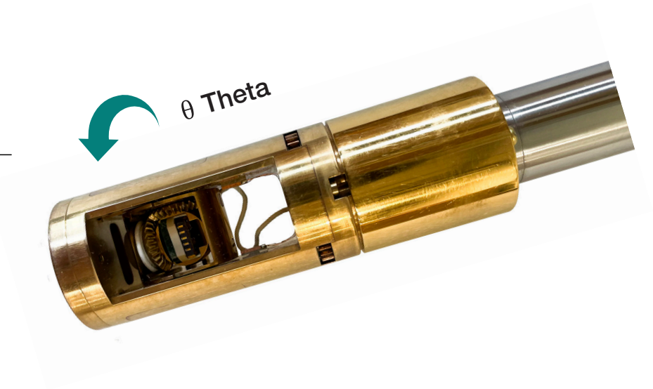
Hall Voltage Measured using a Two Axis Rotator: Theta Sweeps
