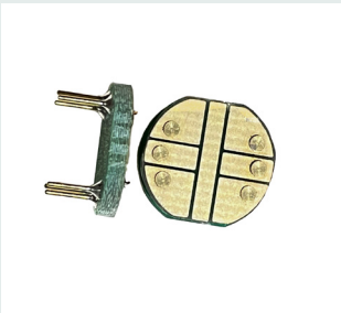
6 pin sample chip and probe end
