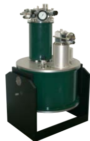
12 Tesla magnet with top loading variable temperature cryostat
